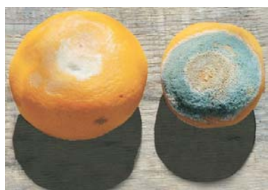
Ozone arrests mould growth (Ozonated sample on the left, control on the right.)
